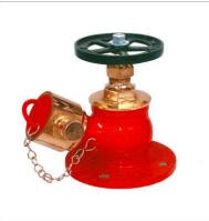
Hydrant valves (also called Landing valves) provide the means to draw water for fire fighting from the Fire water piping network. They are normally mounted onto stand posts, fitted on the fire water network.
